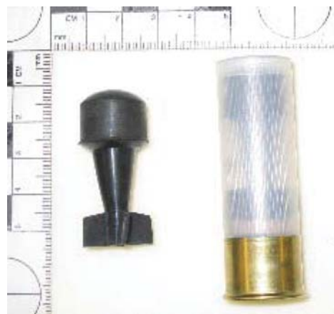
FIG. 3—The 12 gauge, fin-stabilize rubber rocket kinetic energy munition.
